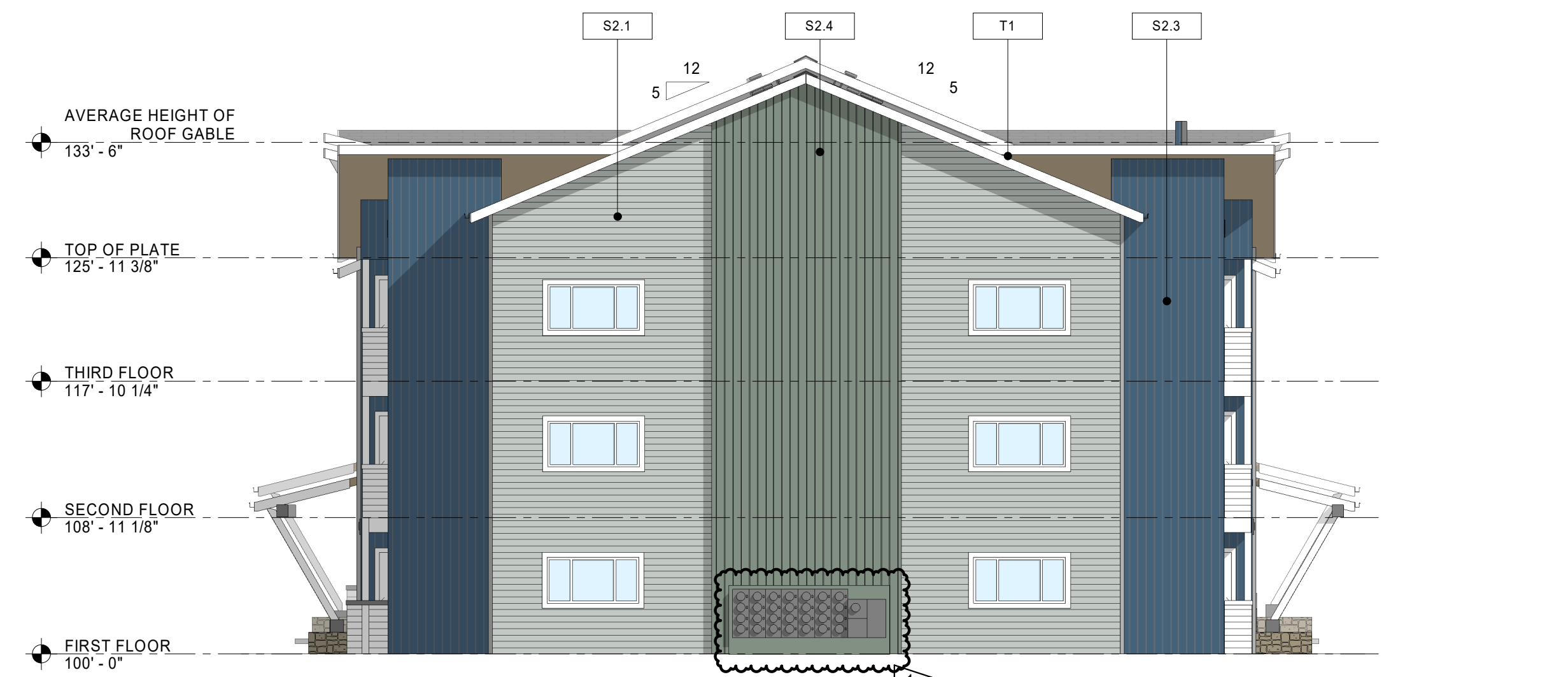
1 BUILDING TYPE 2 - END ELEVATION (NORTH) A5.3 1/8" = 1'-0"
