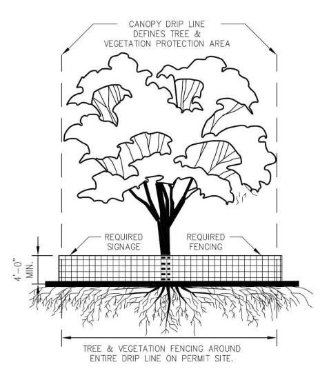
Image 1. An example of a Tree Protection Zone barrier. Contact information of the site manager or consulting arborist should also be included on the sign.
