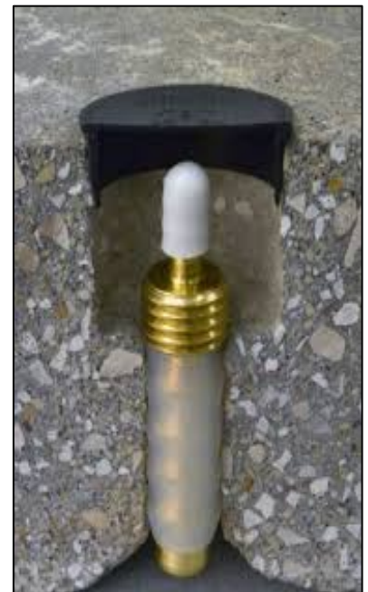
Photo 2. Vapor Pin in Concrete Slab
