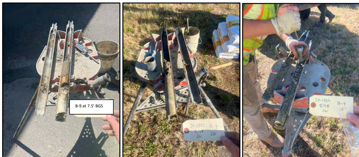
Images 6 (left), 7 (center) and 8 (right) - These images show typical subsurface soil conditions as observed via split spoon sampler at the time of drilling operations in late September of 2024. Image 6 depicts a sandy interbed (advance outwash), that was observed at 7.5 feet BGS, within the glacial till unit. Note the reddish oxidation related to staining and slightly moist conditions above the glacial till contact. Images 7 and 8 illustrate typical glacial till materials (Image 7) and a typical glacial outwash interbed as observed in B-4 at 15 feet BGS.
