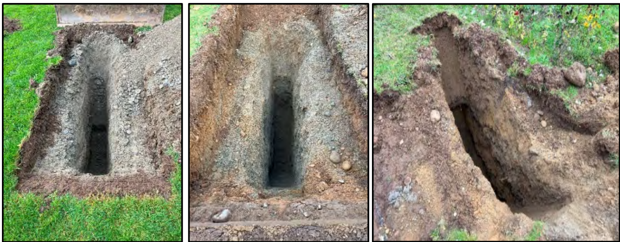
Images 9 (left), 10 (center) and 11 (right) - These images show typical subsurface soil conditions as observed during test pit excavation. Image 9 shows TP-7 and demonstrates conditions consisting of topsoil over glacial till deposits. Image 10 shows TP-1 and illustrates topsoil over weathered trending to unweathered advance outwash deposits. Image 11 shows TP-10 and depicts uncontrolled fill over relict topsoil over weathered trending to unweathered glacial till deposits.
