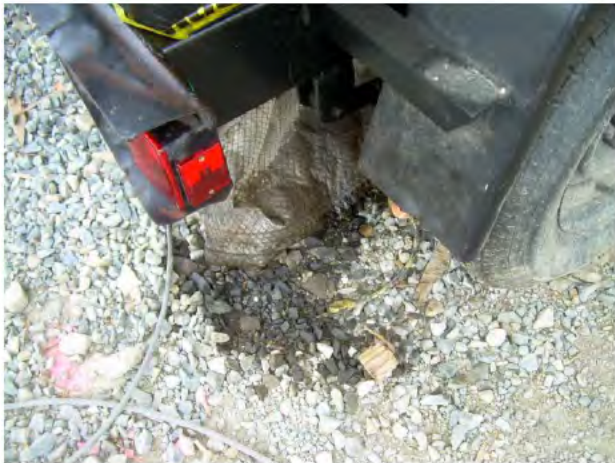
Photo 4-20. Dripping oil from compressor.
