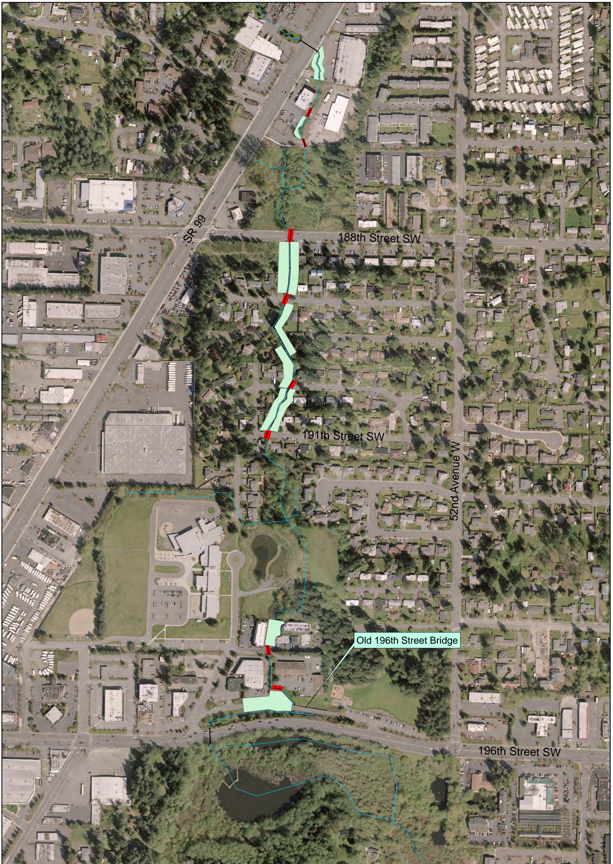
Figure 7 Scriber Creek Flood Reduction Study 196th To 188th Phase 2 Existing Conditions Stream Bank Overtopping Areas
