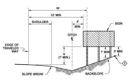
**MULTIPLE SIGN POST INSTALLATION** IN DITCH SECTION
