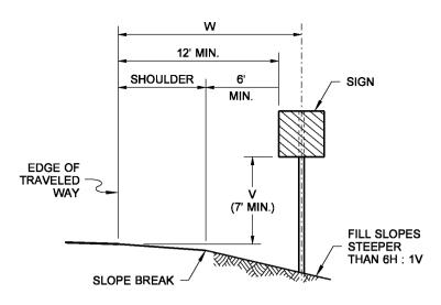
**SIGN INSTALLATION ON STEEP FILL SLOPES**
