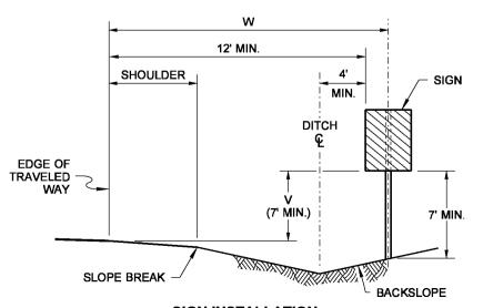
**SIGN INSTALLATION** IN DITCH SECTION
