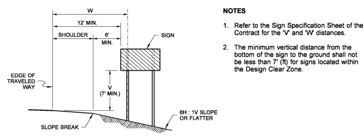
**MULTIPLE SIGN POST INSTALLATION** IN FILL SECTION
