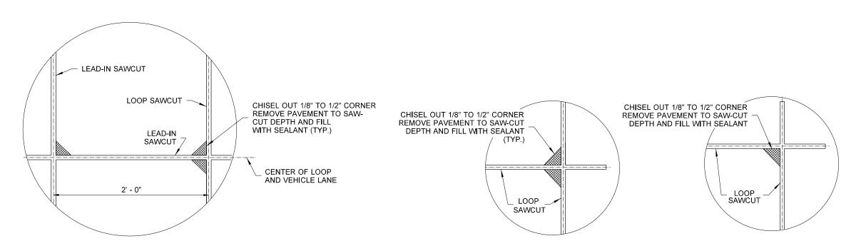
ENTRANCE SAWCUT DETAIL T - SAWCUT DETAIL CORNER SAWCUT DETAIL
