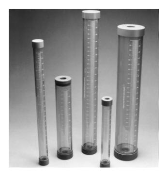
**Griffco** calibration cylinders are designed to enhance the performance of chemical feed systems by providing a verification of the flow rate of the chemical feed pump. Robust construction of clear PVC with an easy to read graduation in mls and gph. Available in three models: EZ-Clean, Vented, and Open Top; and 13 sizes; 100 mL through 20,000 mL as detailed here.
